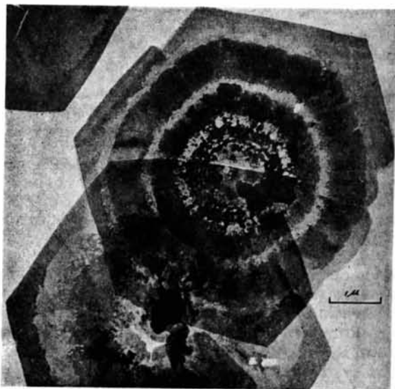
Fig. 1. Electron micrograph of basic lead carbonate particles.
